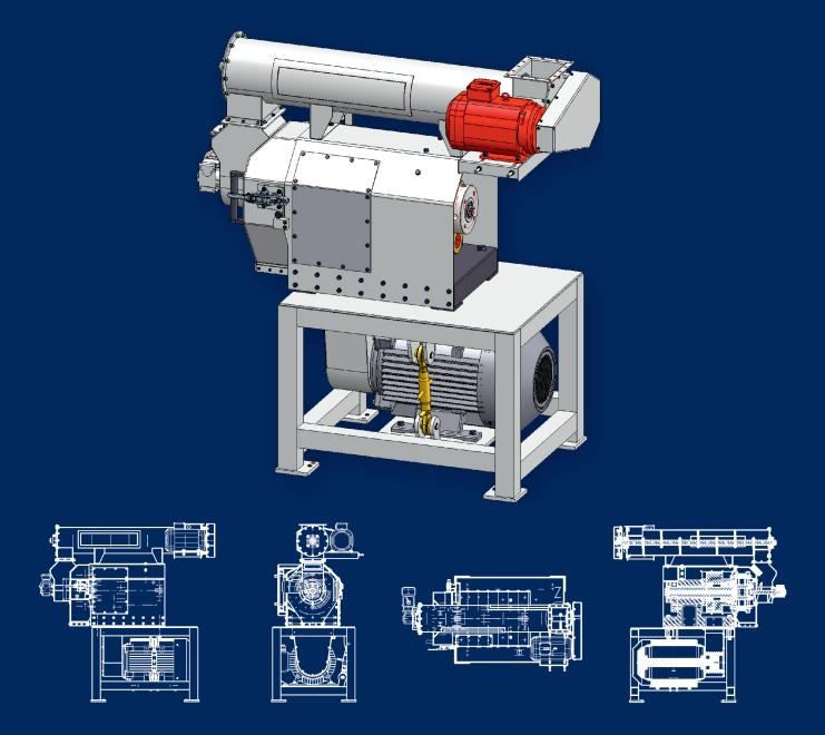
For the palletisation of biomass up to a maximum input moisture content of 15%
